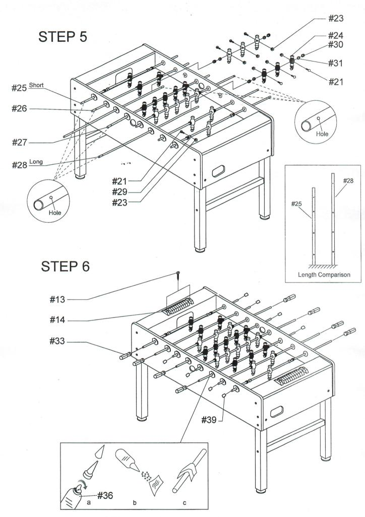
• Spray the lubricant(#36) into a clean, soft cloth and then use the cloth to wipe the player rods where they come into contact with the bearings. See above.
